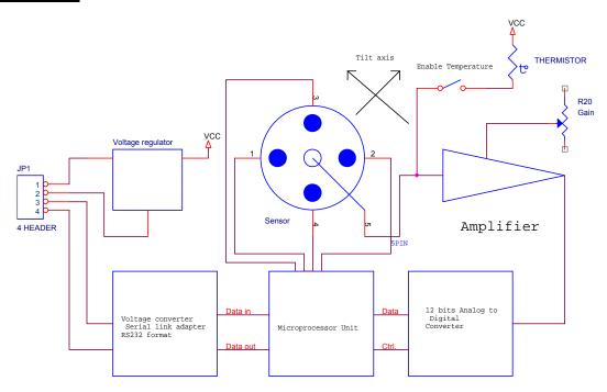
Note . Gain Adjustment is accomplished by adjusting the potentiometer (R20) on the circuit board.
