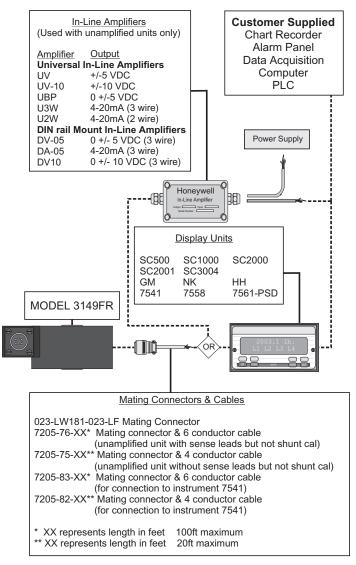
SUNSTAR传感与控制 http://www.sensor-ic.com/ TEL:0755-83376549 FAX:0755-83376182 E-MAIL:szss20@163.com Low Capacity Fatigue Load Cell
