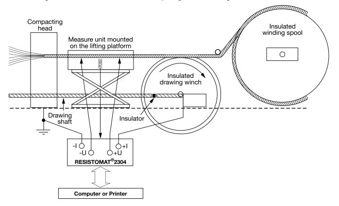
The RESISTOMAT<sup>®</sup> 2304 has not necessarily to be mounted directly at the clamping device 2382 A. The instrument can also be placed at the general control elements of the machine.
