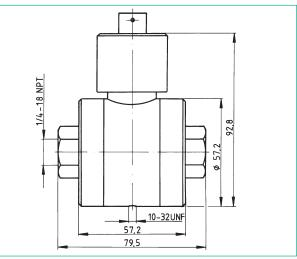
The differential pressure transducers are designed for a line pressure up to 140 bar and are designed for large pressure differences such as occur on double-acting hydraulic cylinders in construction machinery or material test devices. If the measuring range in the positive direction is restricted, the transducers can be used at a higher line pressure - up to the maximum value given in the table.
