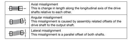
Misalignments interfere with the measurement and should be compensated largely.
