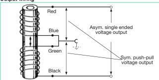
The speed sensors can be operated single ended or with a push-pull output. The wiring connections for each are shown in the drawing. It is also possible to connect them in parallel (connect the red wire to the green, the blue to the black). This reduces the source impedance of the coils to 1/4 and the output voltage to half of the values given in the table above.
