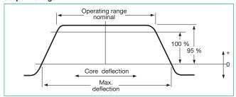
Output voltage based on core deflection, for constant speed.
