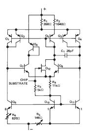
Figure 1. Schematic Diagram
