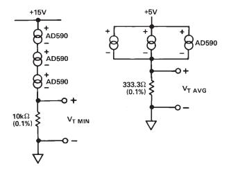
Figure 11. Series & Parallel Connection
