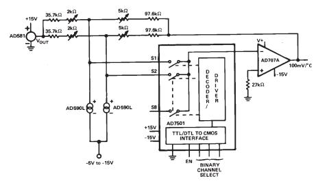
Figure 19. 8-Channel Multiplexer
