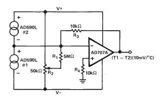
Figure 12. Differential Measurements
