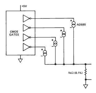
Figure 17. AD590 Driven from CMOS Logic
