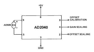
Figure 10. Variable Scale Display
