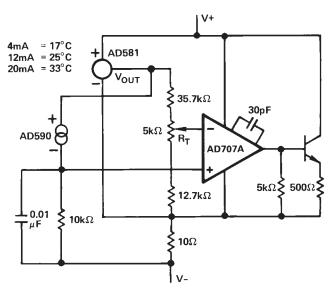
Figure 14. 4 mA-to-20 mA Current Transmitter
