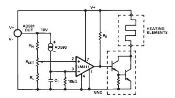
Figure 15. Simple Temperature Control Circuit
