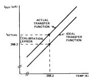
Figure 3. Calibration Error vs. Temperature
