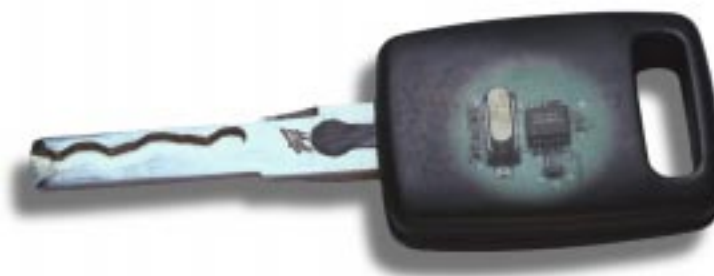
Figure 1 - Single-chip RF-circuits has resulted in a wide range of ingenious wireless systems (Photo courtesy of Jan Meyer)
