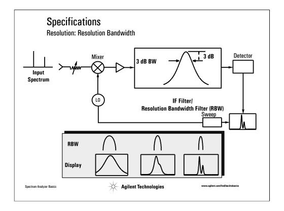
One of the first things to note is that a signal cannot be displayed as an infinitely narrow line. It has some width associated with it. This shape is the analyzer's tracing of its own IF filter shape as it tunes past a signal. Thus, if we change the filter bandwidth, we change the width of the displayed response. Agilent datasheets specify the 3 dB bandwidth. Some other manufacturers specify the 6 dB bandwidth.
