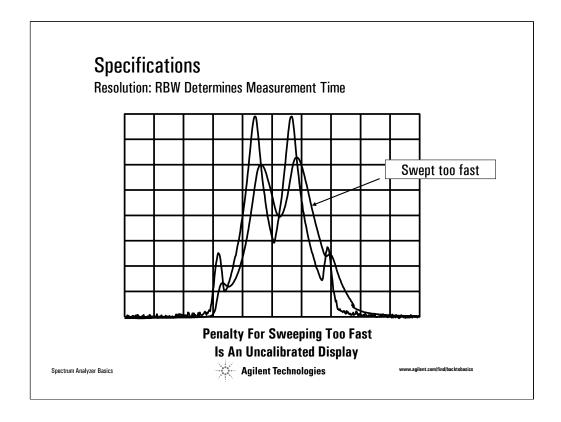
When we narrow the resolution bandwidths for better resolution, it takes longer to sweep through them because they require a finite time to respond fully.
