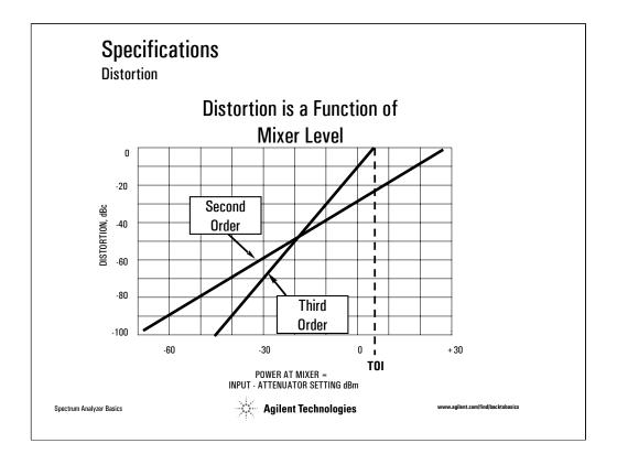
Understanding this concept is useful in determining distortion within the analyzer. Here we plot the level of the secondand third-order distortion products relative to the signals that cause them. The x-axis is the signal power at the first mixer (in this case the level of the tone or tones). The y-axis is the spectrum analyzer's internally- generated distortion level in dBc (dB below the signal level at the mixer). These curves are *signal-to-distortion curves*.
