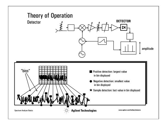
The analyzer must covert the IF signal to a baseband or video signal so it can be digitized and then viewed on the analyzer display. This is accomplished with an envelope detector whose video output is then digitized with an analog-to-digital converter (ADC). The digitized output of the ADC is then represented as the signal's amplitude on the Y-axis of the display. This allows for several different detector modes that dramatically affect how the signal is displayed.
