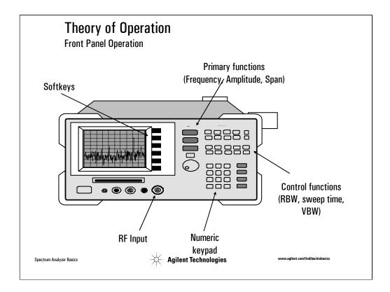
Before we move on, its important to know what we can control on the analyzer via the front panel keys.
