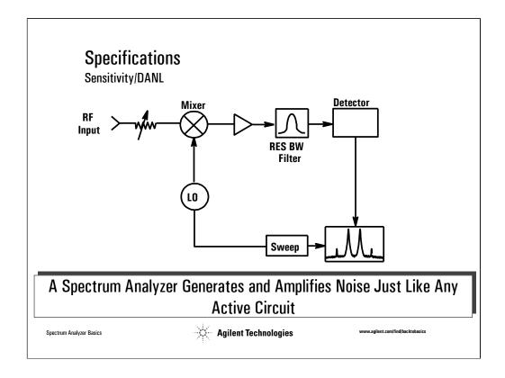
One of the primary uses of a spectrum analyzer is to search out and measure low-level signals. The **sensitivity** of any receiver is an indication of how well it can measure small signals. A perfect receiver would add no additional noise to the natural amount of thermal noise present in all electronic systems, represented by kTB (k=Boltzman's constant, T=temperature, and B=bandwidth). In practice, all receivers, including spectrum analyzers, add some amount of internally generated noise.
