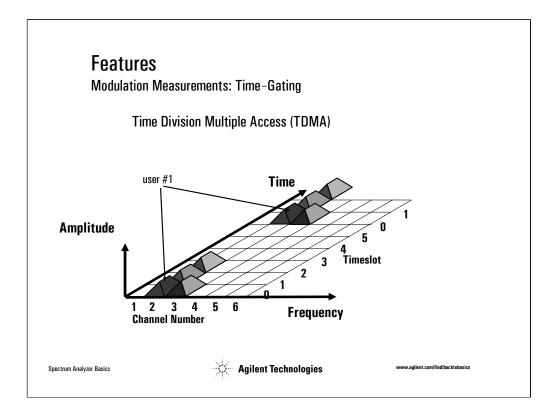
In order to explain the time-gating feature of a spectrum analyzer, we will use a digital communications application, Time-Division-Multiple-Access (TDMA). This is a common method used in communications in order to increase channel capacities in the same frequency bands. TDMA divides up the frequency channels into time slots, so that users can occupy the same frequency, but use different timeslots.
