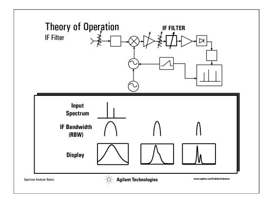
The IF filter is a bandpass filter which is used as the "window" for detecting signals. It's bandwidth is also called the resolution bandwidth (RBW) of the analyzer and can be changed via the front panel of the analyzer.
