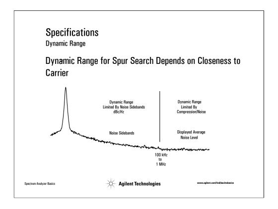
The final factor in dynamic range is the phase noise, or noise sidebands, on our spectrum analyzer LO.
