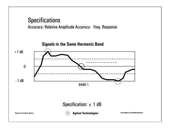
The frequency response, or flatness of the spectrum analyzer, also plays a part in relative amplitude uncertainties and is frequency-range dependent. A low-frequency RF analyzer might have a frequency response of 0.5 dB. On the other hand, a microwave spectrum analyzer tuning in the 20 GHz range could well have a frequency response in excess of 4 dB.
