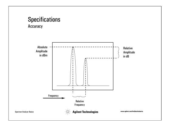
The second area to understand is **accuracy**; how accurate will my results be in both frequency and amplitude? When talking about accuracy specifications, it is important to understand that there is both an absolute accuracy specification, and a relative accuracy specification.
