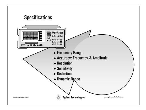
What do you need to know about a spectrum analyzer in order to make sure you choose one that will make your particular measurements, and make them adequately? Very basically, you need to know 1) what's the frequency range? 2) what's the amplitude range (maximum input and sensitivity)? 3) to what level can I measure the difference between two signals, both in amplitude (dynamic range) and frequency (resolution)? and 4) how accurate are my measurements once I've made them?
