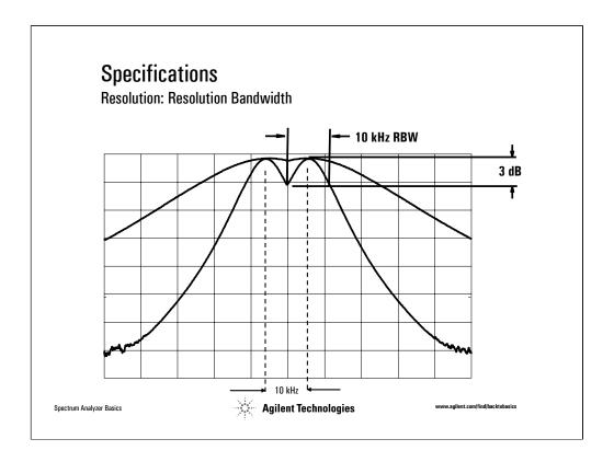
When measuring two signals of equal-amplitude, the value of the selected RBW tells us how close together they can be and still be distinguishable from one another (by a 3 dB 'dip').
