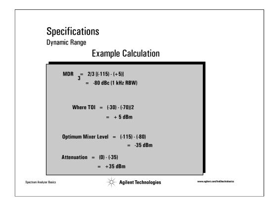
For example, let's say we have a spectrum analyzer with a DANL = -115 dBm (1 kHz RBW), and TOI = +5 dBm. This slide shows how to calculate maximum third-order dynamic range (MDR<sub>3</sub>), optimum mixer level, and attenuation.
