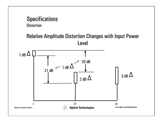
Most distortion measurements are made relative to the fundamental signals (the carrier or two-tones). When the fundamental power is decreased 1 dB, the second-order distortion decreases by 2 dB, but relative to the fundamental, the second-order distortion decreases 1 dB. There is a one-for-one <u>relative</u> relationship between the fundamental and second-order distortion.
