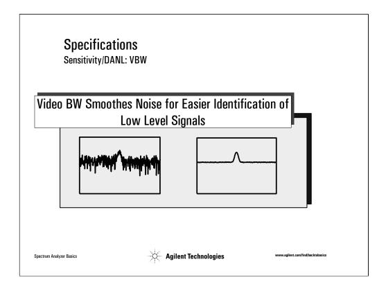
In the Theory of Operation section, we learned how the video filter can be used to smooth noise for easier identification of low level signals. Since we are talking about measuring low level signals, we will repeat it here. The VBW, however, does not affect the frequency resolution of the analyzer (as does the RBW), and therefore changing the VBW does not improve sensitivity. It does, however, improve discernability and repeatability of low signal-to-noise ratio measurements.
