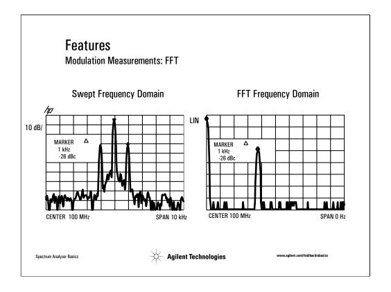
Another common measurement made on an AM signal (besides determining the modulation frequency) is modulation index, which tells us the degree of modulation (0 to 100%).
