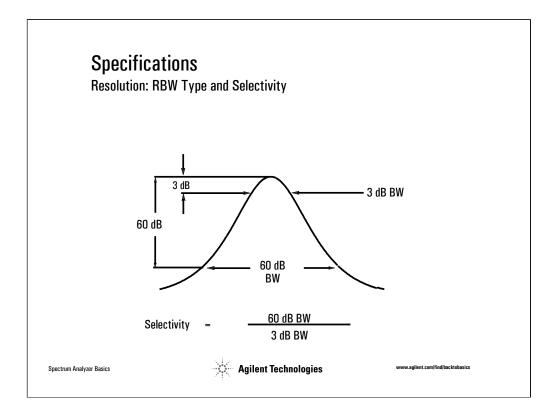
Selectivity is the important characteristic for determining the resolvability of unequal amplitude signals.
