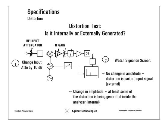
Before leaving this section on distortion, there is a test that should be done for all distortion measurements. The test is going to tell us whether or not what we are seeing on the screen is internally generated distortion, or distortion caused by the DUT.
