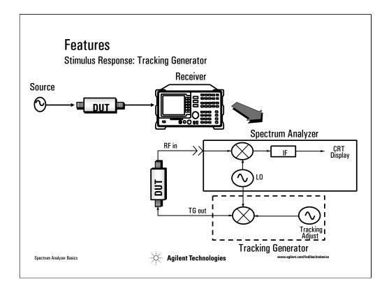
Stimulus response measurements, which are also called network measurements, is where we apply a signal to the input of our device/system and measure the response at the output.
