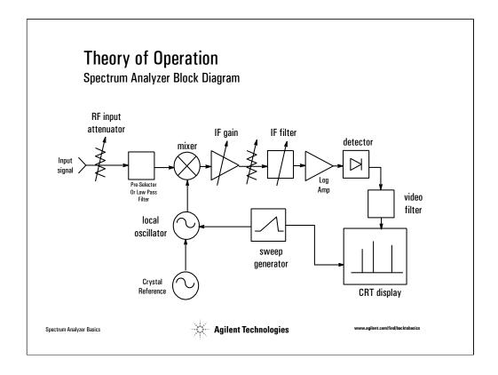
The major components in a spectrum analyzer are the RF input attenuator, mixer, IF (Intermediate Frequency) gain, IF filter, detector, video filter, local oscillator, sweep generator, and LCD display. Before we talk about how these pieces work together, let's get a fundamental understanding of each component individually.
