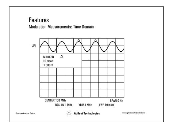
It was mentioned briefly that although a spectrum analyzer is primarily used to view signals in the frequency domain, it is also possible to use the spectrum analyzer to look at the time domain. This is done with a feature called zero-span. This is useful for determining modulation type or for demodulation.
