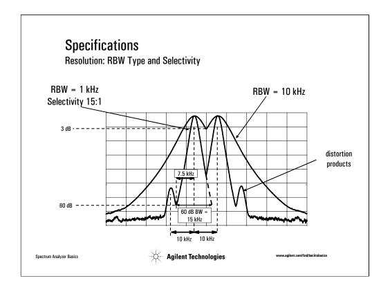
For example, say we are doing a two-tone test where the signals are separated by 10 kHz. With a 10 kHz RBW, resolution of the equal amplitude tones is not a problem, as we have seen. But the distortion products, which can be 50 dB down and 10 kHz away, could be buried.
