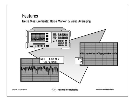
When making measurements on noise, there are a couple of features on a spectrum analyzer that can make the measurements easier and more accurate.
