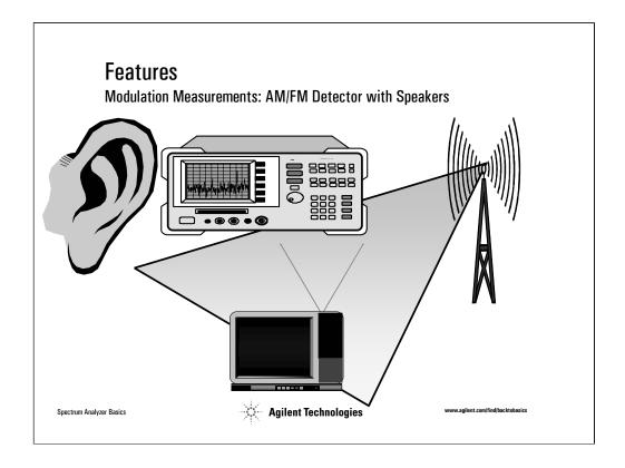
Most modern spectrum analyzers have available AM/FM detection with speakers. The built-in AM/FM detectors with speaker allow you to hear the modulation. In other words, they allow you to hear the source of interference as well as see it, for faster identification of interfering signals in communication networks, etc.
