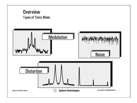
The most common spectrum analyzer measurements are: modulation, distortion, and noise.
