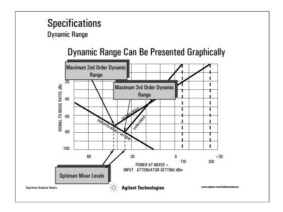
Let's plot both the signal-to-noise and signal-to-distortion curves on one dynamic range graph. *Maximum dynamic range* occurs where the curves intersect, that is, when the internally generated distortion level equals the displayed average noise level. This shows two of the dynamic range specifications. We will see that there are others later.
