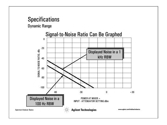
On page 54, we plotted the signal-to-distortion curves. This graph is actually called a dynamic range graph, and just as we plotted distortion products as a function of mixer power, we can also plot *signal-to-noise ratio* (SNR) as a function of mixer power.
