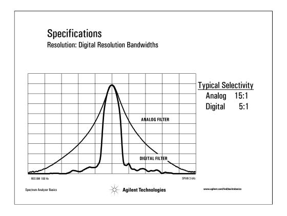
One thing to note before we close the topic of resolution is that Digital RBWs (i.e. spectrum analyzers using digital signal processing (DSP) based IF filters) have superior selectivity and measurement speed. The following table illustrates this point. For example, with a 100 Hz RBW, a digital filter is 3.1 times faster than an analog.
