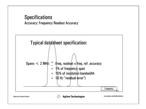
Frequency accuracy is often listed under the Frequency Readout Accuracy specification and is usually specified as the sum of several sources of errors, including frequency-reference inaccuracy, span error, and RBW center-frequency error.
