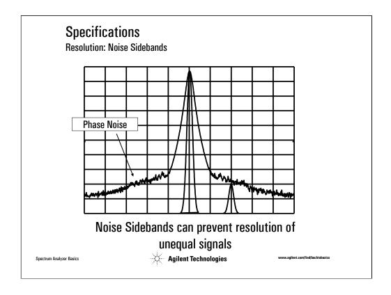
The remaining instability appears as *noise sidebands* (also called phase noise) at the base of the signal response. This noise can mask close-in (to a carrier), low-level signals that we might otherwise be able to see if we were only to consider bandwidth and selectivity. These noise sidebands affect resolution of close-in, low-level signals.
