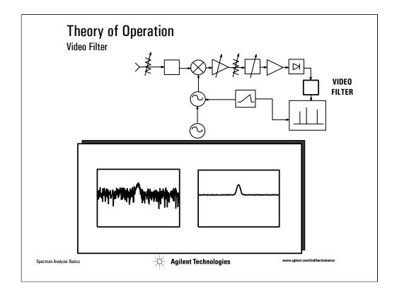
The video filter is a low-pass filter that is located after the envelope detector and before the ADC. This filter determines the bandwidth of the video amplifier, and is used to average or smooth the trace seen on the screen.
