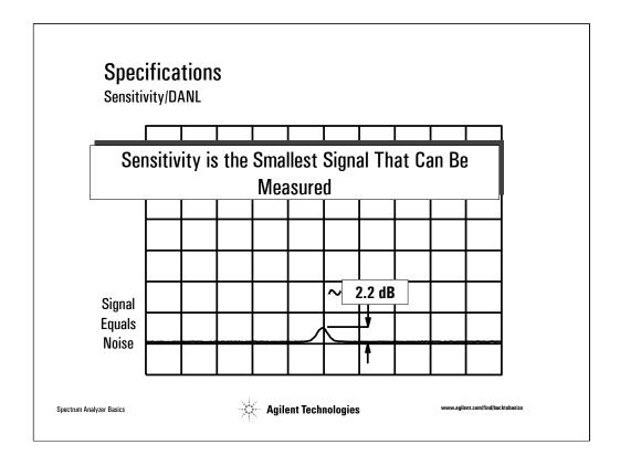
A signal whose level is equal to the displayed average noise level (DANL) will appear approximately as a 2.2 dB bump above the displayed average noise level. This is considered to be the minimum measurable signal level. However, you won't be able to see this signal unless you use video filtering to average the noise.
