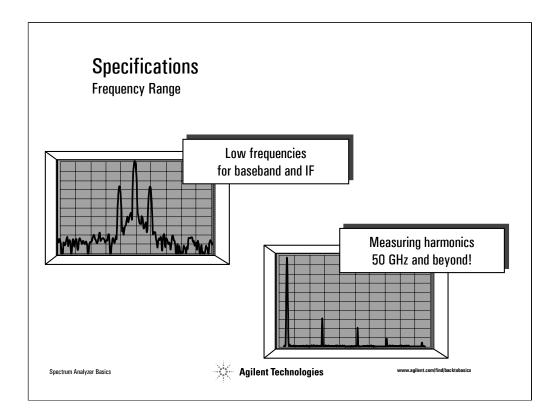
Of course, the first and foremost specification you want to know is the **frequency range** of the analyzer. Not only do you want a spectrum analyzer that will cover the fundamental frequencies of your application, but don't forget harmonics or spurious signals on the high end, or baseband and IF on the low end.
