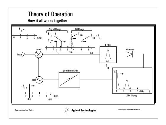
Let's put it all together now. Note that while the RF input attenuator, IF gain, and video filter are important, they are not critical when describing how the analyzer works.
