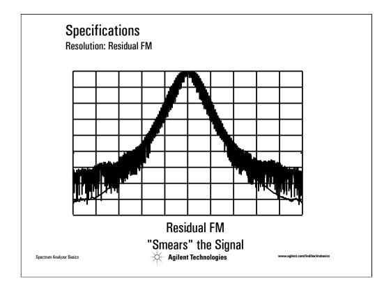
Another factor affecting resolution is the frequency stability of the spectrum analyzer's local oscillator. This inherent short-term frequency instability of an oscillator is referred to as residual FM. If the spectrum analyzer's RBW is less
