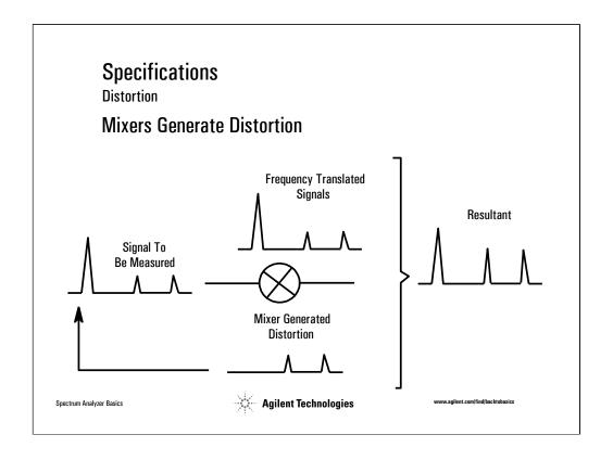
Although distortion measurements, such as third order intermodulation and harmonic distortion, are common measurements for characterizing devices, the spectrum analyzer itself will also produce distortion products, and potentially disturb your measurement.
