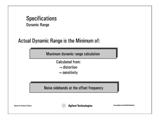
We have seen that the dynamic range of a spectrum analyzer is limited by three factors: the broadband noise floor (sensitivity) of the system, the distortion performance of the input mixer, and the phase noise of the local oscillator. The first two factors are used to calculate maximum dynamic range. Therefore, actual dynamic range is the minimum of 1) the MDR calculation and 2) the noise sidebands.
