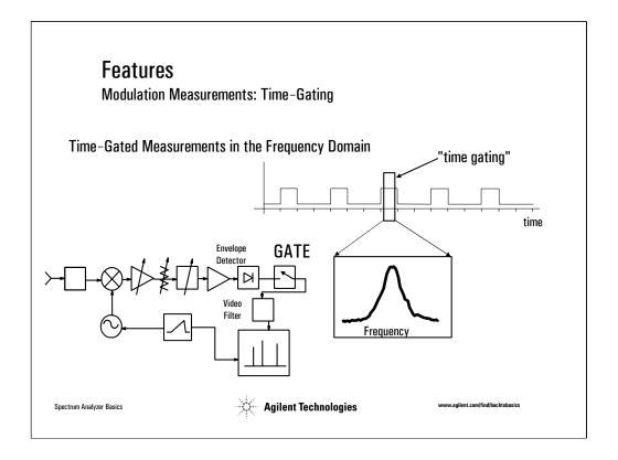
Time-gated, or time-selective spectrum analysis offers a solution to measurement difficulties in the time and frequency domains. Time gating permits precise yet flexible control of the point at which a time domain sweep begins, allowing the sweep to be centered over the desired timeslot. Any timeslot, or portion of a timeslot, may be examined at maximum time resolution.
