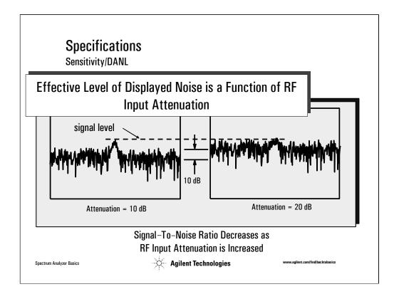
One aspect of the analyzer's internal noise that is often overlooked is its effective level as a function of the RF input attenuator setting.
