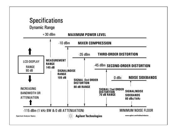
There are several ranges associated with the spectrum analyzer. Typically the term "dynamic range" only refers to the ability to measure two signals at the same time.
