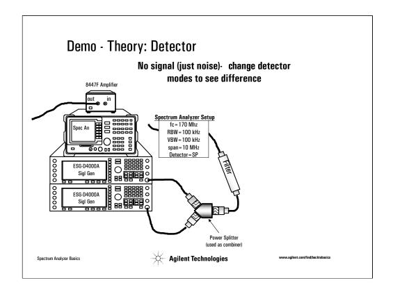
Disconnect signal from analyzer
