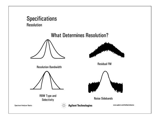
**Resolution** is an important specification when you are trying to measure signals that are close together and want to be able to distinguish them from each other. We saw that the IF filter bandwidth is also known as the resolution bandwidth (RBW). This is because it is the IF filter bandwidth and shape that determines the resolvability between signals.
