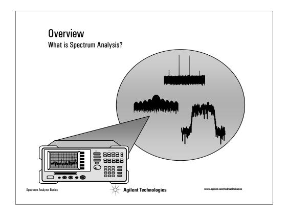
If you are designing, manufacturing, or doing field service/repair of electrical devices or systems, you need a tool that will help you analyze the electrical signals that are passing through or being transmitted by your system or device. By analyzing the characteristics of the signal once its gone through the device/system, you can determine the performance, find problems, troubleshoot, etc.
