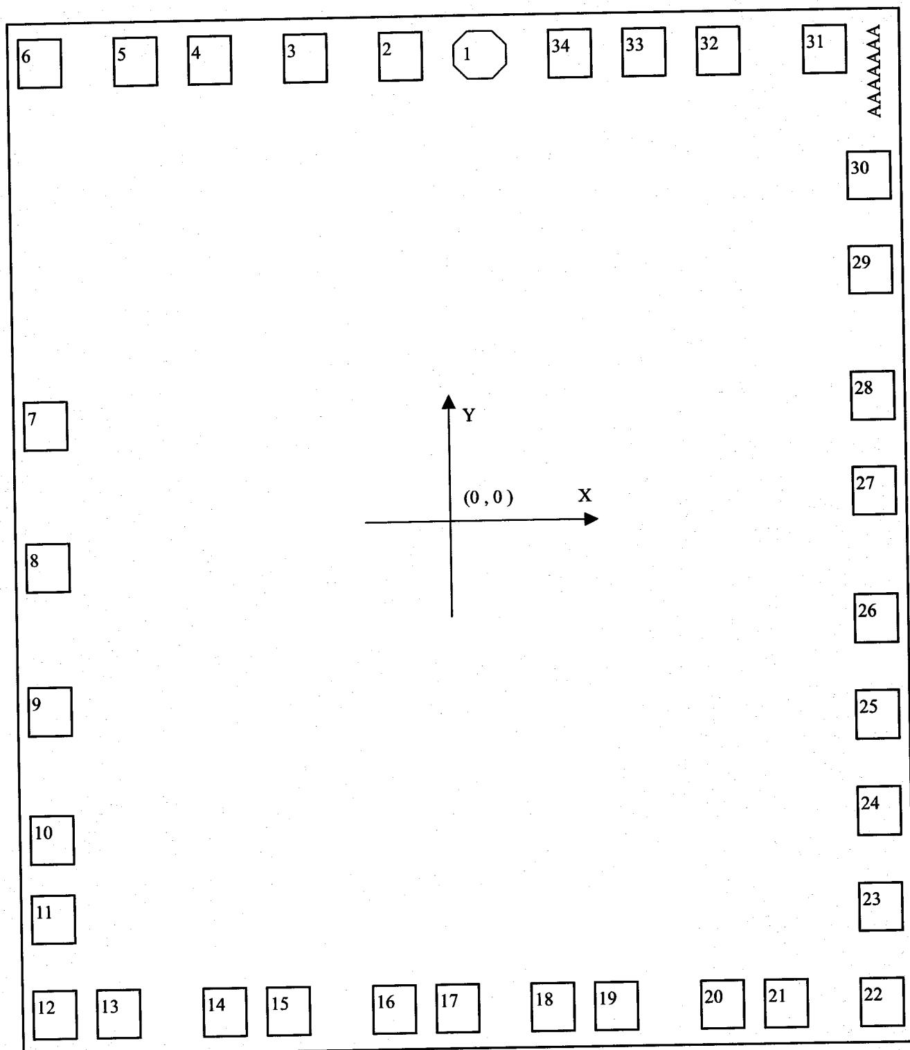
**Chip Size:** (2490\*2750)  $\mu^2$ m   **Note:** The substrate must be connected to VDD.
