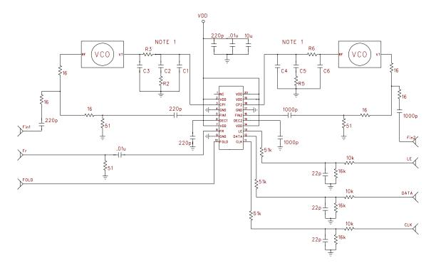
**Note 1:** For optimum fractional spur and lock-time performance  $C_2$  and  $C_5$  should be polyester (or poly propylene). In addition, the loop filter components must be free from contamination. Contamination will result in poor spur performance.
