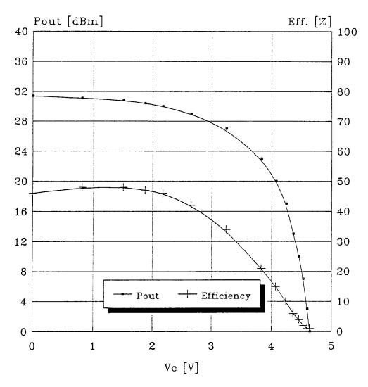
F=900Mhz, Pin=0 dBm, Vs=6V
