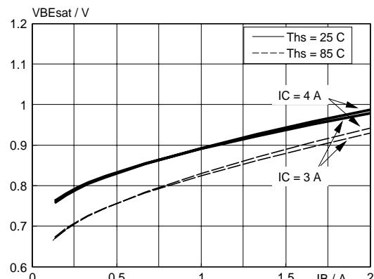
Fig.7. Typical base-emitter saturation voltage.
