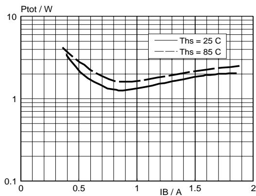
Fig.8. Typical losses.
