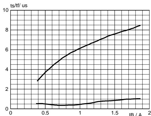
Fig.9. Typical collector storage and fall time.
