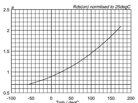
Fig.9. Normalised drain-source on-state resistance.
