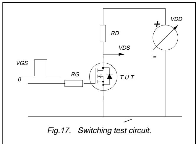
*Fig.17. Switching test circuit.*
