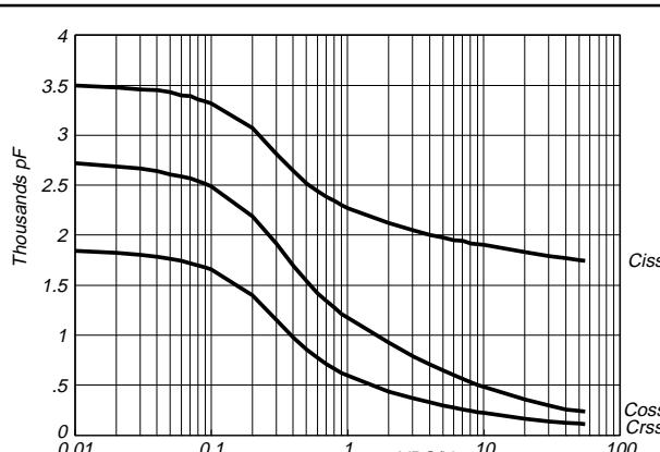
Fig.12. Typical capacitances,  $C_{iss}$ ,  $C_{oss}$ ,  $C_{rss}$ .
