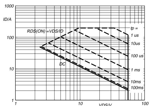
Fig.3. Safe operating area.  $T_{mb} = 25^\circ\text{C}$
