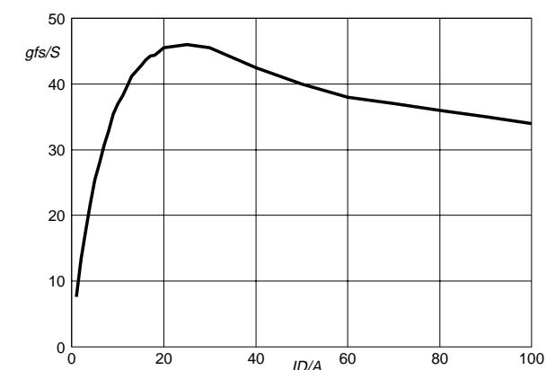
Fig.8. Typical transconductance,  $T_j = 25^\circ\text{C}$ .
