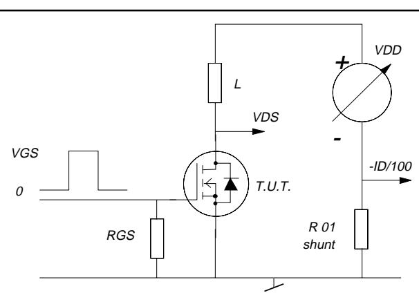
Fig.16. Avalanche energy test circuit.
