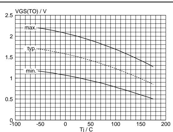
Fig.10. Gate threshold voltage.
