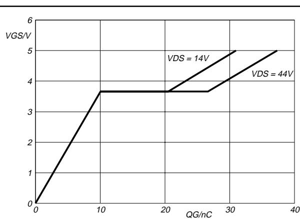
Fig.13. Typical turn-on gate-charge characteristics.
