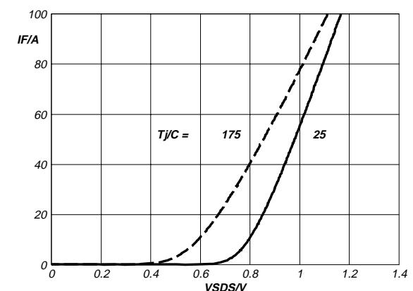
Fig.14. Typical reverse diode current.
