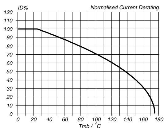
Fig.2. Normalised continuous drain current.
