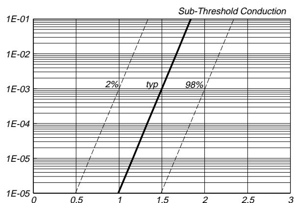
Fig.11. Sub-threshold drain current.
