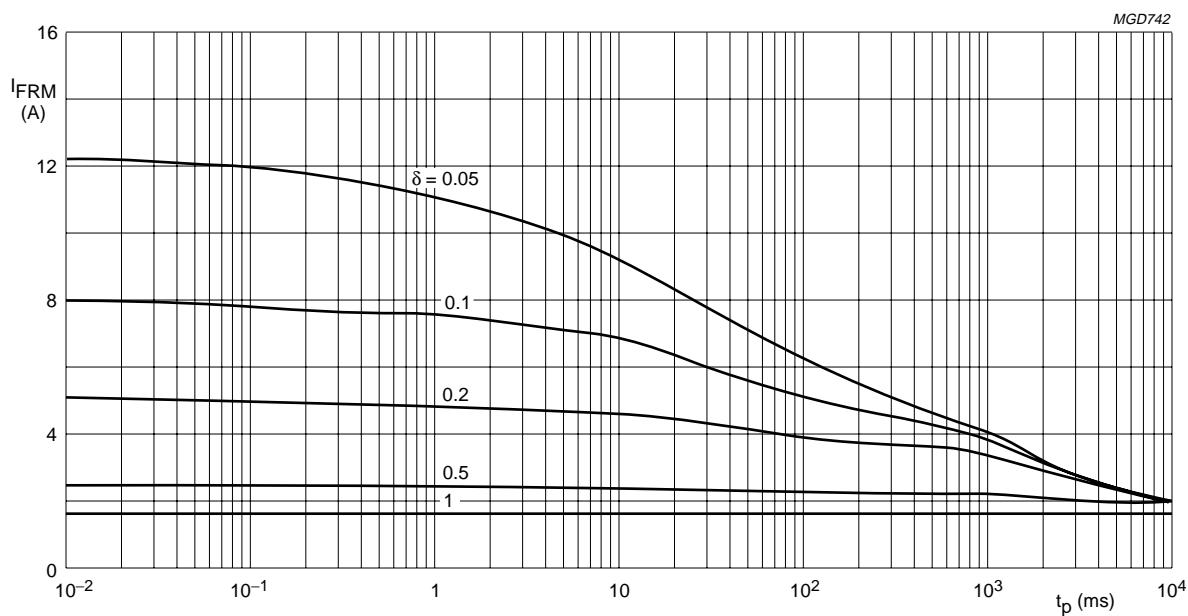
$T_{amb} = 60^\circ\text{C}$ ;  $R_{th\ j\cdot a} = 100 \text{ K/W}$ ;  $V_R = V_{RRMmax}$  during  $1 - \delta$ .
