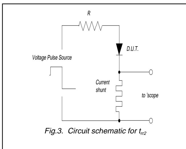
Fig.3. Circuit schematic for  $t_{rr2}$
