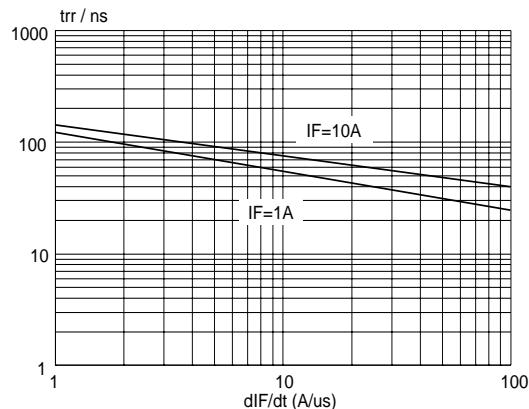
Fig.7. Maximum  $t_{rr}$  at  $T_j = 25^\circ\text{C}$ ; per diode
