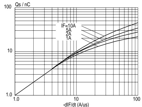
Fig.10. Maximum  $Q_s$  at  $T_j = 25^\circ\text{C}$ ; per diode
