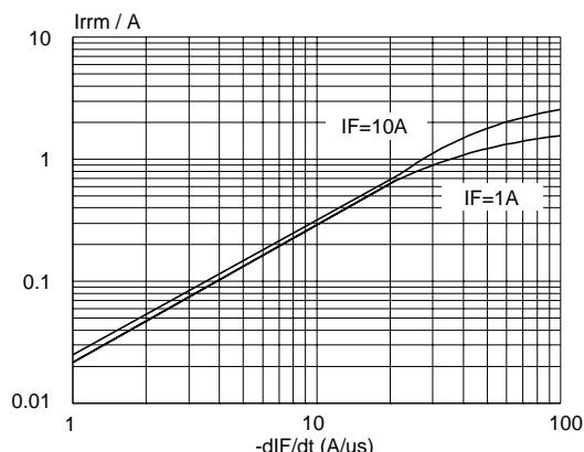
Fig.8. Maximum  $I_{rm}$  at  $T_j = 25^\circ\text{C}$ ; per diode
