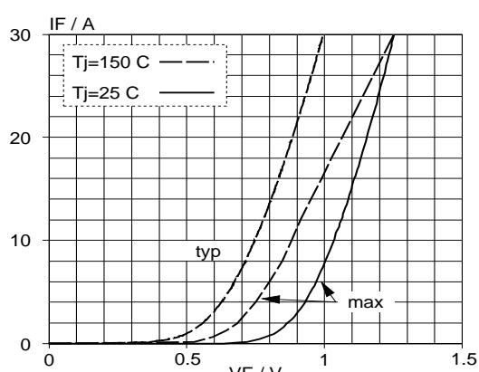
Fig.9. Typical and maximum forward characteristic
