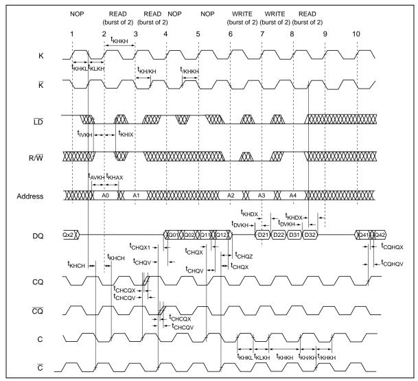
Notes: 1. Q01 refers to output from address A0. Q02 refers to output from the next internal burst address following A0, etc.
