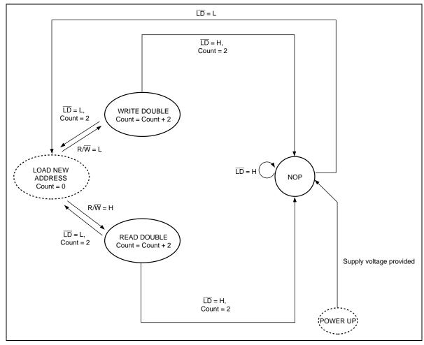
Notes: 1. SA0 is internally advanced in accordance with the burst order table. Bus cycle is terminated after burst count = 2.
