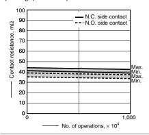
3-(2). Change in static contact resistance (10  $\mu$ A 1 mV DC resistive load) Tested sample: ASX20012, 10 pcs. Operating speed: 750 cpm
