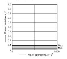
2-(2). Change in dynamic contact resistance (10 µA 1 mV DC resistive load)
