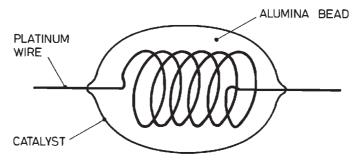
The design has been modified to reduce the amount of power used by the sensor and to make the sensor more resistant to poisoning and mechanical shock. SGX, when known as E2V, was in the forefront of these developments and the current range of pellistors incorporates the design improvements.
