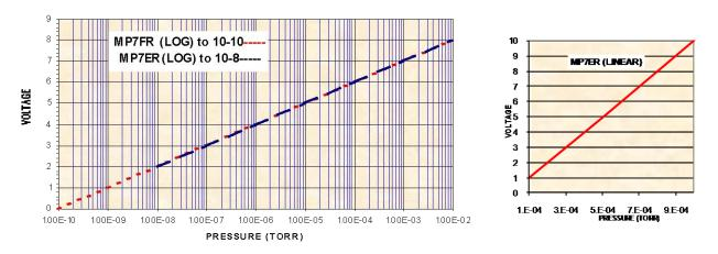
No maintenance is required beyond periodic cleaning or replacement of a contaminated sensor. The 7ER is cleanable whereas the 7FR requires sensor replacement.
