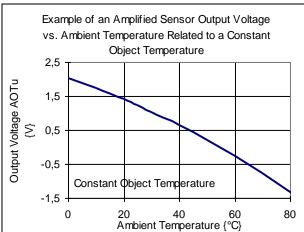
The integrated sensor module HTIA is designed to detect the housing temperature and to convert the temperature to a voltage.
