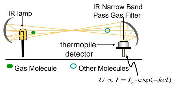
The gas concentration can be measured by monitoring the absorption of an infrared light beam. The base equation for gas concentration measurement in the infrared way is Beer's law:
