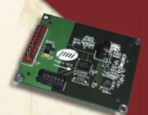
The TCM2.5 is a replacement for PNI's original TCM2 family of products. It offers improved accuracy and performance for compass heading, tilt and magnetometer measurements. It is the same size, has the same 10-pin RS-232 interface connector and is compatible with the original TCM2 ASCII protocol. These features make the TCM2.5 the choice for existing applications that require compatibility the TCM2 family of products.
