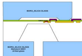
Cross-section of SM5112 Back port hole is 0.8 mm. Silicon is 0.4 mm; top and bottom glass is 0.5 mm
