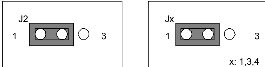
Figure 3.11. Memory Mask Jumpers (J1 to J4)
