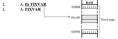
If an odd address is specified, then the data word starting at the even address immediately below it will be accessed (—word boundary).
