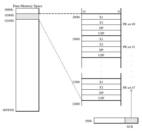
The pointing register set to be used is selected by the SCB field in the PSW. The following table shows the relation between SCB field values and the pointing register set selected. Immediately after reset, pointing register set #0 will be selected. The initial values of all pointing registers are undefined.
