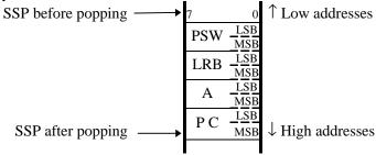
2)Under the small/compact memory models, the PSW, LRB, A, PC, and CSR are popped from the system stack in that order.
