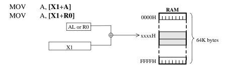
If an odd address is specified, then the data word starting at the even address immediately below it will be accessed (->word boundary).
