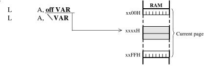
If an odd address is specified, then the data word starting at the even address immediately below it will be accessed ( $\rightarrow$ word boundary).
