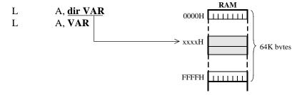
If an odd address is specified, then the data word starting at the even address immediately below it will be accessed (—word boundary).
