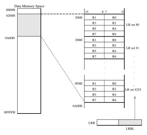
The local register set to be used is selected by the low byte of LRB (LRBL). The starting address of the local register set selected is given by LRBL $\times$  8 + 200H. Immediately after reset, the value of LRBL is undefined, so there is no way to tell which local register set is selected. The initial values of all local registers are undefined.
