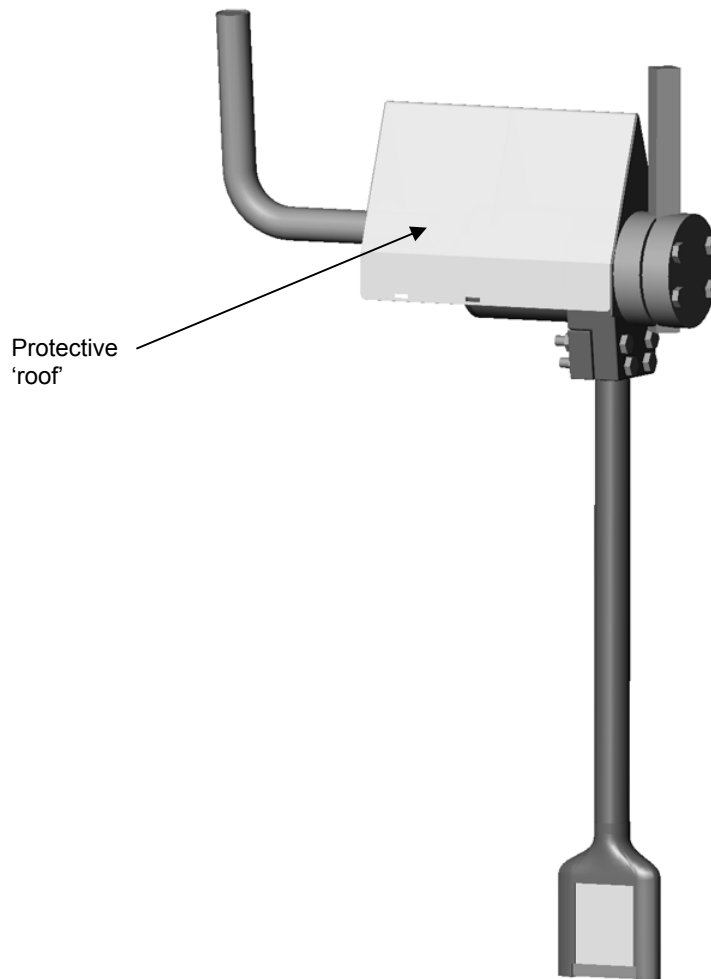
Figure 5 - Protective 'roof' placed over the sensor body
