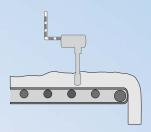
In a rotating pan mixer or conveyor application, the Hydro-Probe Orbiter can be cabled directly to the control system. In a static pan mixer the sensor cable is routed through the Hydronix Rotating Connector.
