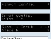
Tare in , Tare out , Set zero, Printou active (new Data, Alibi, print) Repeat printout active Interlock1: only Terminal mode. Interlock2: 'Setup' not allowed. Keep output value at Slot 1or2
