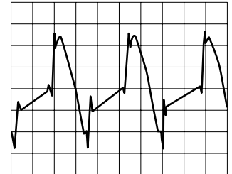
Voltage between SG to output terminals 0.1V/div, 0.5μs/div
