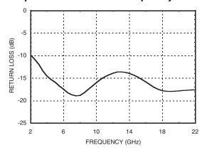
Note: Measured Performance Characteristics (Typical Performance at 25°C) Vd=2.0 V, Id=55 mA
