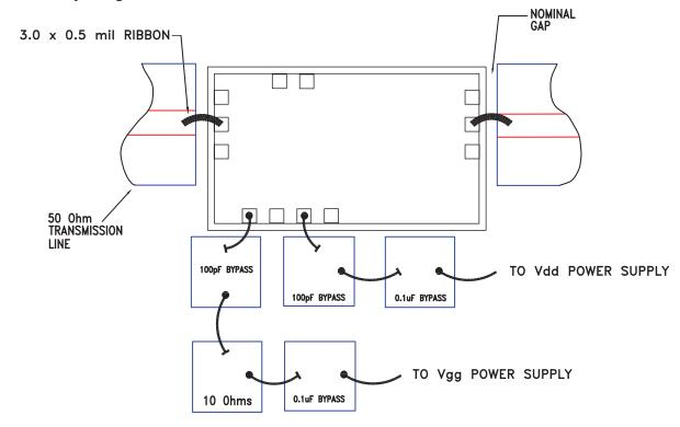
Note 1: Bypass caps should be 100 pF (approximately) ceramic (single-layer) placed no farther than 30 mils from the amplifier.
