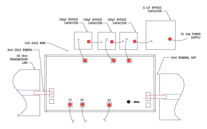
Note: G1, G2 and G3 must be connected to RF/DC ground.
