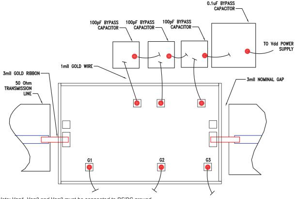
Note: Vgg1, Vgg2 and Vgg3 must be connected to RF/DC ground.
