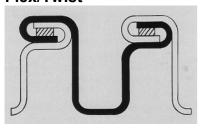
Flexible/Twistable is sealed electrically via a friction joint. This construction has the best twistable performance of all TWS waveguides. The Twistable waveguide core will hold limited pressure, but relies on the jacket for pressure sealing. Flex/Twist is not recommended for low PIM applications -use TWS seamless core.
