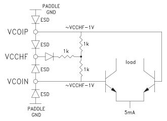
Figure 11. RF Input Stage
