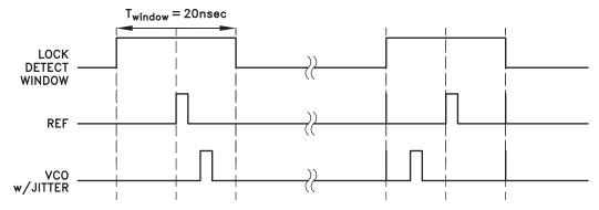
Figure 21. Normal Lock Detect Window
