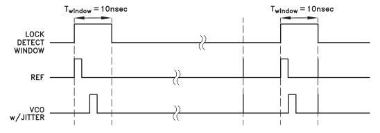
Figure 22. Delayed Lock Detect Window
