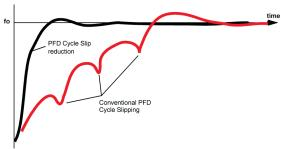
Figure 23. Cycle Slip Prevention (CSP)
