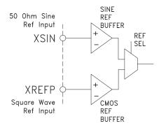
Figure 7. Reference Sine Input Stages
