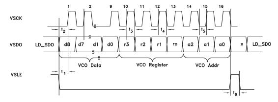
Figure 31. VCO Serial Port Timing Diagram - WRITE ONLY
