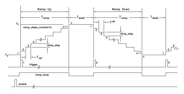
Figure 26. 2-Way Sweep Control via Trigger
