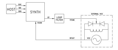
Figure 15. Conventional Synthesizer with VCO
