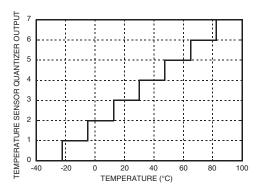
Figure 19. Typical Temperature Sensor Quantizer output
