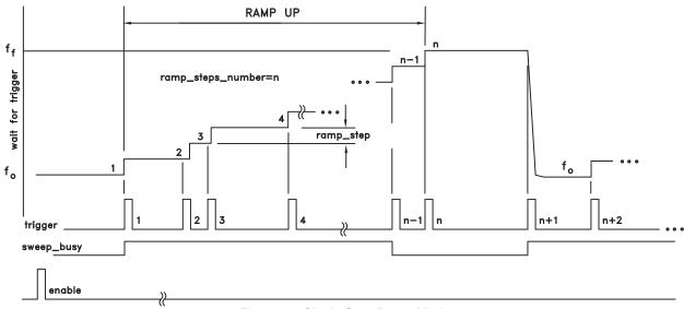
Figure 28. Single Step Ramp Mode
