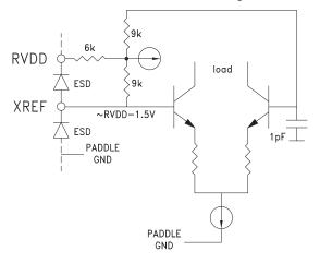
Figure 9. Square Wave Ref Input Stage
