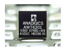
The module requires only the most basic interconnects. All the RF ports are 50 ohms. The power control interfaces directly with the baseband power
