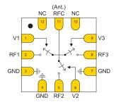
The AWS5533 is a SP3T RF switch developed for CDMA systems. Manufactured in ANADIGICS state-of-the-art pHEMT process, the device uses patent-pending circuit topologies to provide the low insertion loss, high port-to-port isolation and high linearity needed to enhance the performance of CDMA wireless handset radios.
