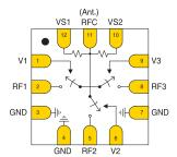
The AWS5523 is a single pole three throw (SP3T) RF switch designed to meet the stringent requirements of GSM systems. Manufactured in ANADIGICS state-of-the-art pHEMT process, the device uses patent-pending circuit topologies to provide the low insertion loss, high port-to-port isolation and high linearity needed to enhance the performance of GSM wireless handset radios.
