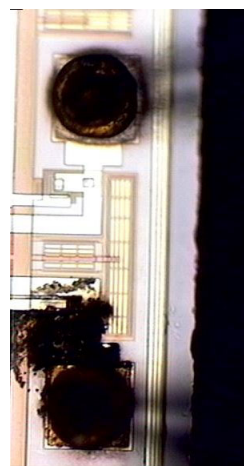
Figure 5. Burn mark on Competitor ‘A’ parts
