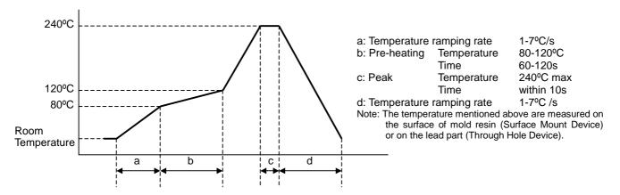
3) Soldering Temperature Profile of Iron
