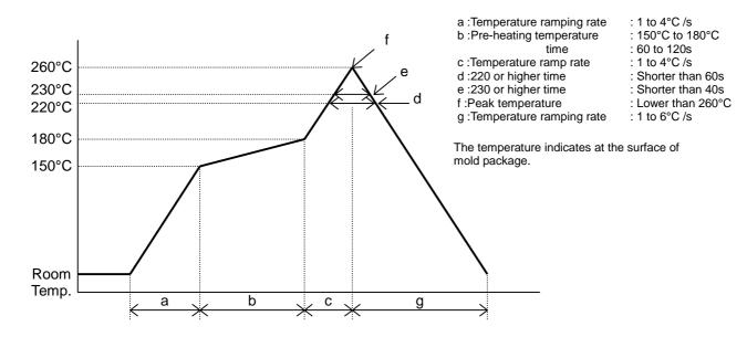
2) Soldering Temperature Profile of Flow Recommended flow soldering temperature profile is in the following.
