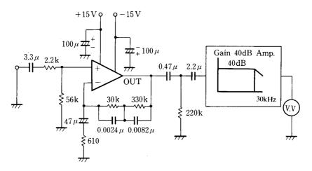
Noise Voltage (Flat+JIS A) measurement Circuit
