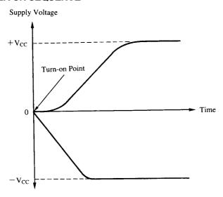
It is necessary that the IC is always used in the condition of no floating GND terminal. Therefore, it is necessary to be noted on using the dual power supply as follows;
