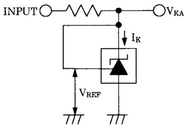
1,  $V_{KA} = V_{REF}$
