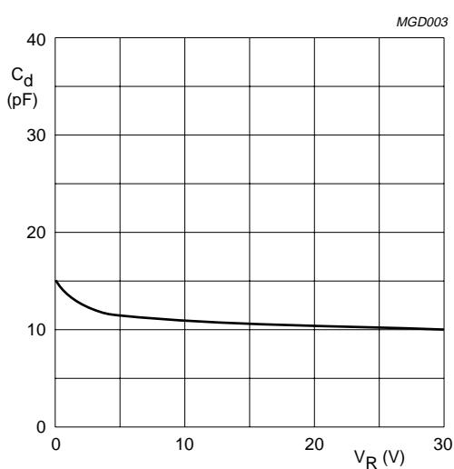
$f = 1 \text{ MHz}; T_j = 25 \text{ }^{\circ}\text{C.}$
