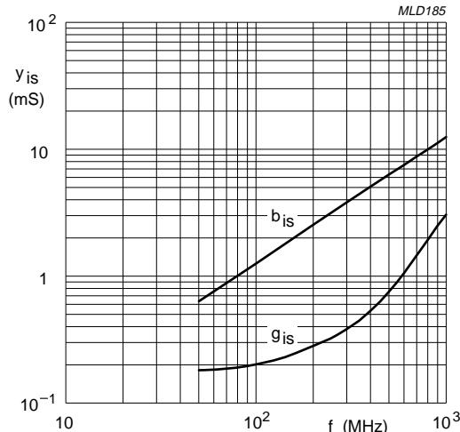
$V_{DS} = 12$  V;  $V_{G2} = 4$  V.
