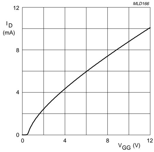
$V_{DS} = 12$  V;  $V_{G2-S} = 4$  V.
