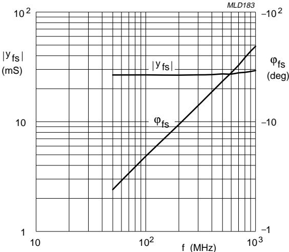
$V_{DS} = 9$  V;  $V_{G2} = 4$  V.
