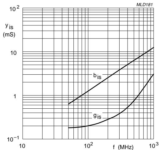
$V_{DS} = 9$  V;  $V_{G2} = 4$  V.
