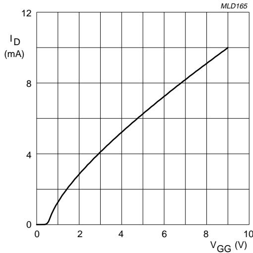
$V_{DS} = 9$  V;  $V_{G2-S} = 4$  V.
