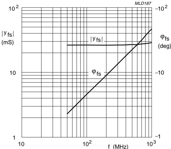
$V_{DS} = 12$  V;  $V_{G2} = 4$  V.
