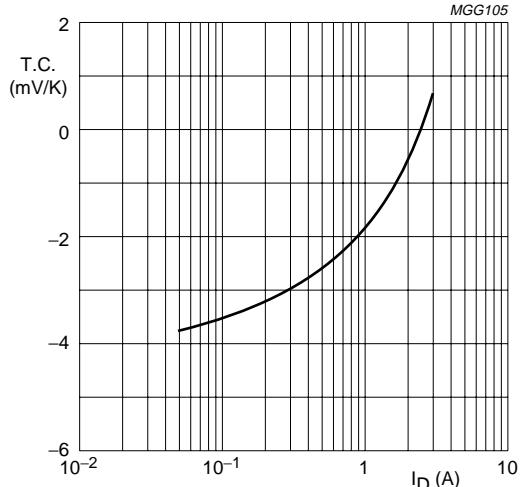
$V_{\text{DS}} = 10 \text{ V}$ ; valid for  $T_h = 25$  to  $70^\circ\text{C}$ .
