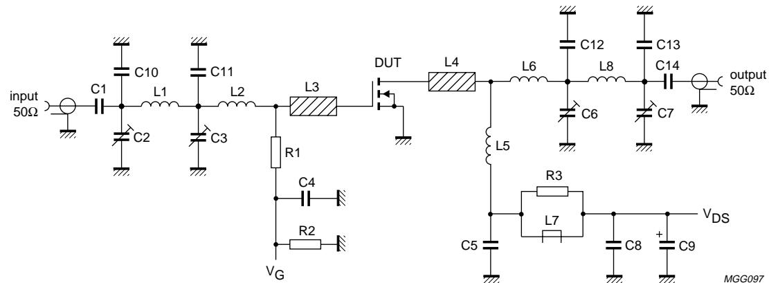
Fig.11 Test circuit for class-B operation at 108 MHz.
