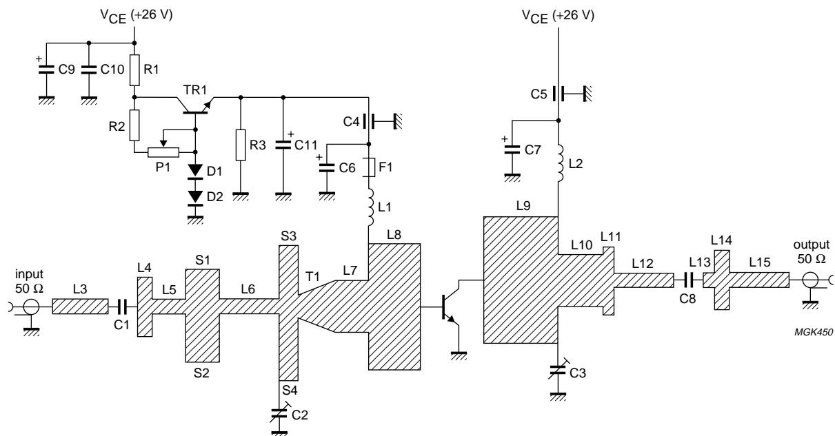
Fig.8 Class-AB test circuit for 1990 MHz.
