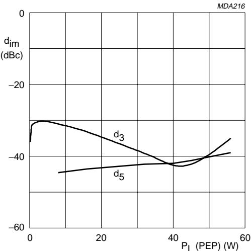
$V_{CE} = 26$  V;  $I_{CQ} = 200$  mA;  $f_1 = 1990$  MHz;  $f_2 = 1990.1$  MHz.
