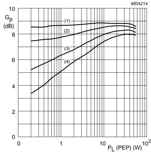
$V_{CE} = 26$  V;  $f_1 = 1990$  MHz;  $f_2 = 1990.1$  MHz.
