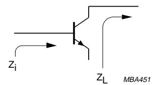
Fig.13 Definition of transistor impedance.
