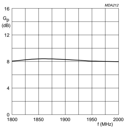
$V_{CE} = 26$  V;  $I_{CQ} = 200$  mA;  $P_L = 50$  W;  $T_{mb} = 25$  °C.
