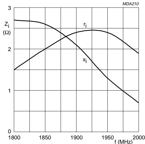
$V_{CE} = 26$  V;  $I_{CQ} = 400$  mA;  $P_L = 50$  W;  $T_{mb} = 25$  °C.
