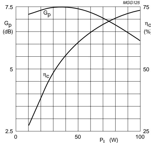
$V_{CE} = 28$  V;  $I_{C(ZS)} = 0.1$  A;  $T_h = 70$  °C;  $f_{vision} = 224.25$  MHz.
