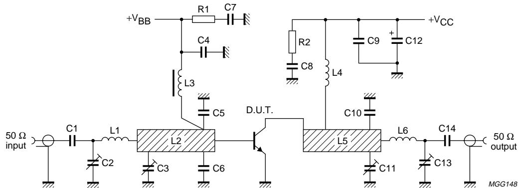
Fig.9 Class-A test circuit at  $f_{\text{vision}} = 224.25$  MHz.
