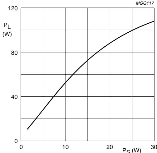
$V_{CE} = 28$  V;  $I_{C(ZS)} = 0.1$  A;  $T_h = 70$  °C;  $f_{vision} = 224.25$  MHz.
