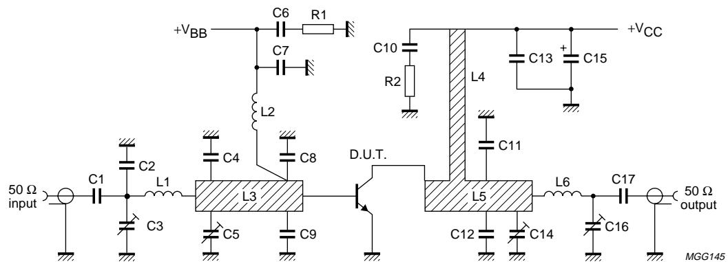
Fig.16 Class-AB test circuit at  $f_{vision} = 224.25$  MHz.
