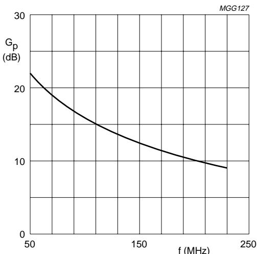
Class-A operation;  $V_{CE} = 25$  V;  $I_C = 3.2$  A;  $T_h = 70$  °C.
