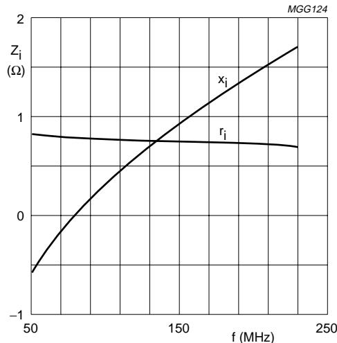
Class-AB operation;  $V_{CE} = 28$  V;  $P_L = 80$  W (PEP);  $T_h = 70$  °C.
