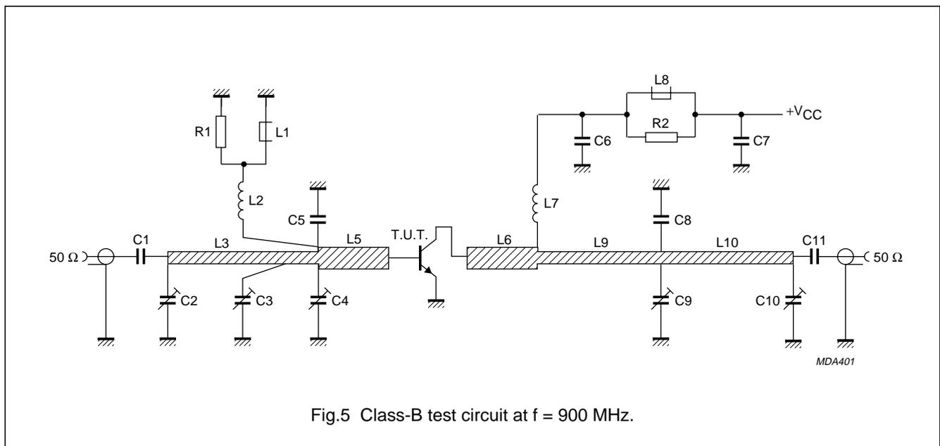
Fig.5 Class-B test circuit at  $f = 900 \text{ MHz}$ .
