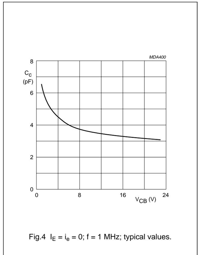
Fig.4  $I_E = i_e = 0; f = 1\text{ MHz}$ ; typical values.
