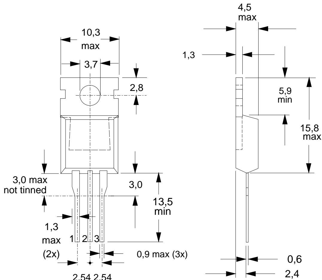
Fig.13. TO220AB; pin 2 connected to mounting base.
