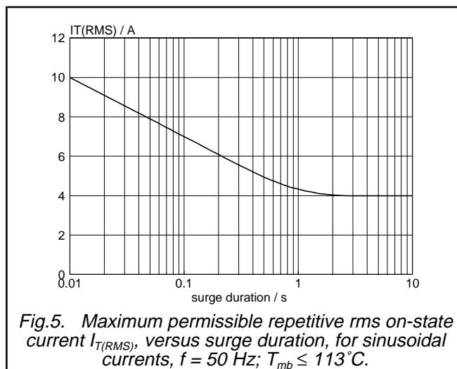
Fig.5. Maximum permissible repetitive rms on-state current  $IT_{(RMS)}$ , versus surge duration, for sinusoidal currents,  $f = 50$  Hz;  $T_{mb} \leq 113^\circ\text{C}$ .
