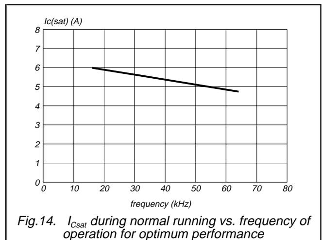
Silicon Diffused Power Transistor
