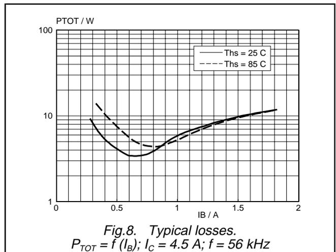
Silicon Diffused Power Transistor
