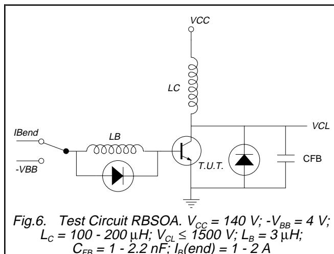
Fig.6. Test Circuit RBSOA.  $V_{CC} = 140$  V;  $-V_{BB} = 4$  V;  $L_C = 100 - 200 \mu\text{H}$ ;  $V_{CL} \leq 1500$  V;  $L_B = 3 \mu\text{H}$ ;  $C_{FB} = 1 - 2.2 \text{ nF}$ ;  $I_B(\text{end}) = 1 - 2 \text{ A}$
