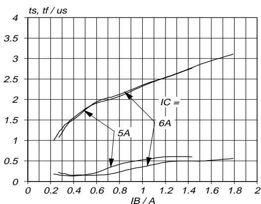
Fig.12. Typical collector storage and fall time.
