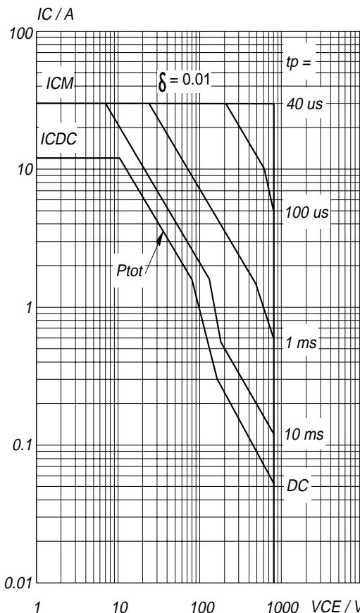
Fig.15. Forward bias safe operating area.  $T_{mb} = 25^\circ C$
